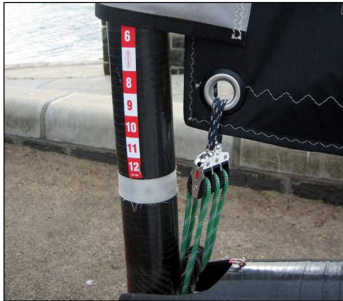
Downhaul set right for maximum upwind boat speed in around 18 knots of wind.
